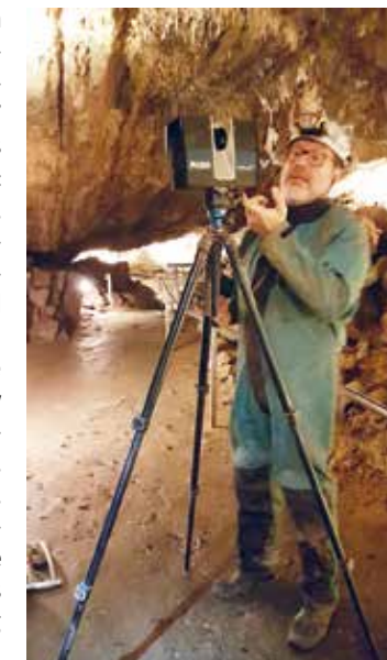
installation of the Faro lidar scanner.
